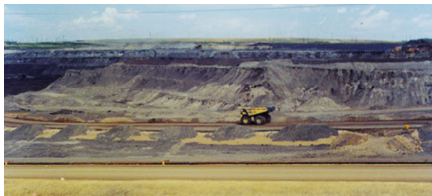
Fig. 21.2 Athabasca tar sand. The oil-impregnated sand is mined and the heavy oil is separated from the sand with hot water
