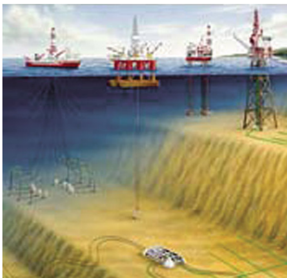
Fig. 17.18 Permanent installation of 4C cables at the sea bottom over a producing field. It improves data quality by ensuring more accurate receiver locations within the repeated 3D surveys over a period of time
