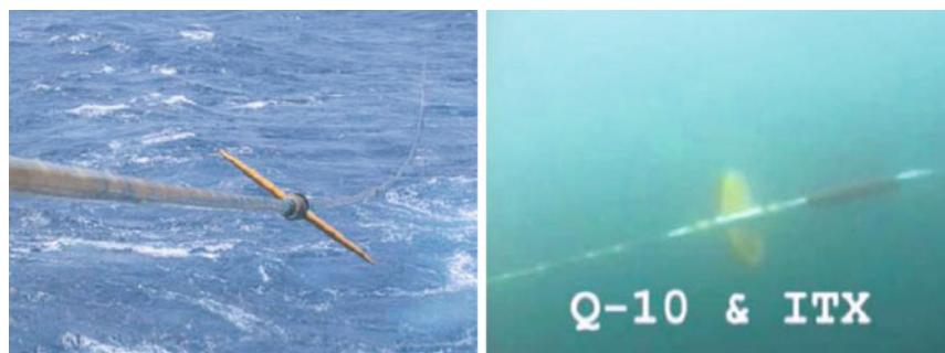
Fig. 19.14 Photographs of the birds (controlling devices) attached to a marine seismic cable at deployment ( left ) and in water operation ( right ). These devices make it possible to steer the cable with reasonable accuracy into a given position (Courtesy of WesternGeco)
