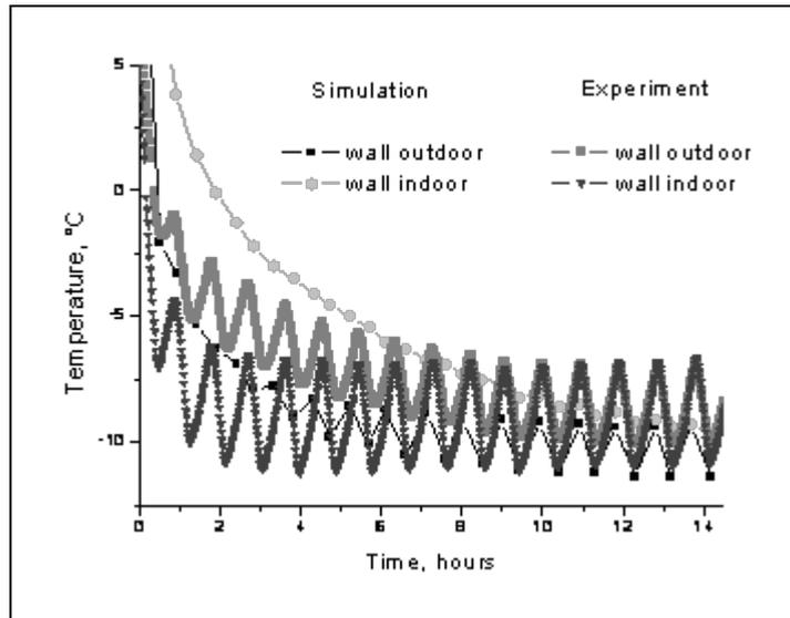
**Fig. 13. The experimentally measured temperature time series and the ones calculated using heat flux time series.**
