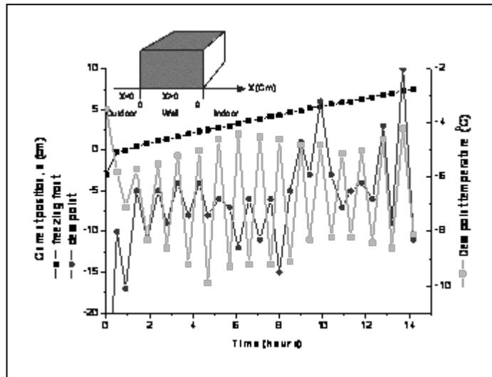
**Fig. 12. Dew point and freezing front coordinate time dynamics.**
