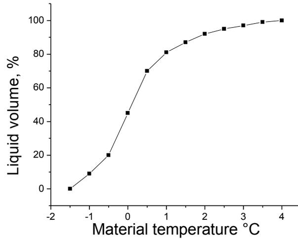
**Fig. 1. Liquid volume fraction dependency on material temperature.**
